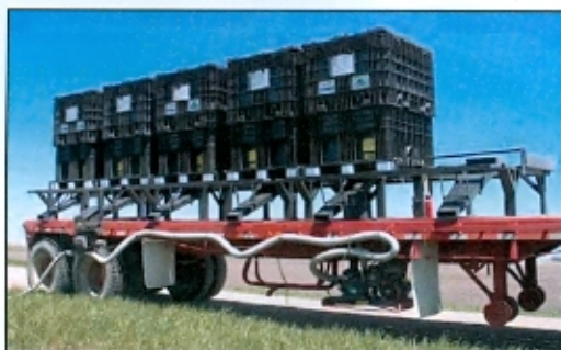
Figure 4: Semi flatbed with power unit below deck
