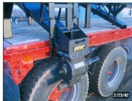
Figure 3: Rolling Bracket with Q-bit Adapter and Air Lock
